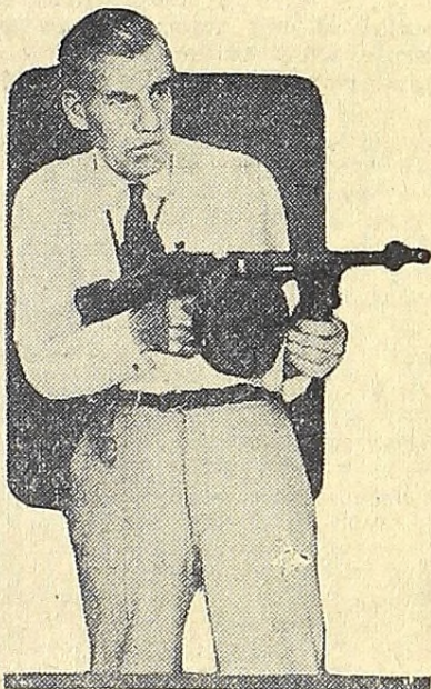
Hector Fuller is here holding a Thompson submachine gun at the Bankers' Industrial exposition in New York. The baby machine gun weighs but nine pounds thirteen ounces, but is capable of "spitting" a stream of 300 bullets a minute.
