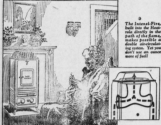
built into the Heat-rola directly in the path of the flame, makes possible a double air-circulating system. Yet you don't use an ounce more of fuel!
