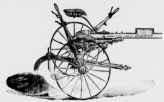
A High Lift, Light Draft; Easily Backed Sulky, incapable of being tipped over; fitted with foot trip engaging with the power lift, also foot guide for regulating width of farrow and plowing around curves.
