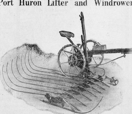
Teasily and quickly attached to any mower without removing any bolts or drilling any holes. Most efficient attachment on the market for harvesting seed peas or clover seed; suitable for harvesting any down or tangled grain, such as Alfalfa, Lucerne, Buckwheat, Timothy, etc. ¶Large savings can be made by use of the lifter in gathering green peas for canning purposes.
